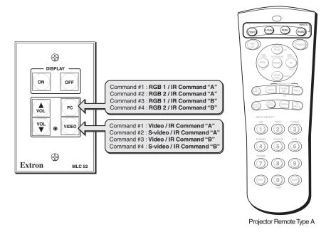
Programming MLC 52 input selection buttons from a projector remote control type A
